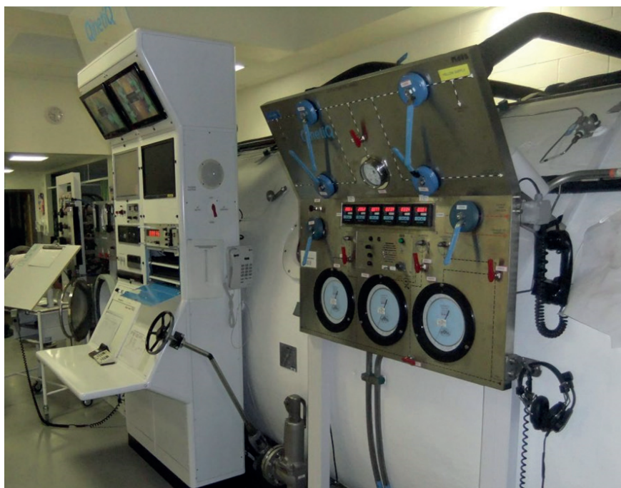
Figure 1: A modified Royal Navy recompression chamber which can be pressurised to an equivalent depth of 85 metres below sea level (reproduced from www.uhsussex.nhs.uk/services/hyperbaric-medicine/ with kind permission of University Hospitals Sussex NHS Foundation Trust).
